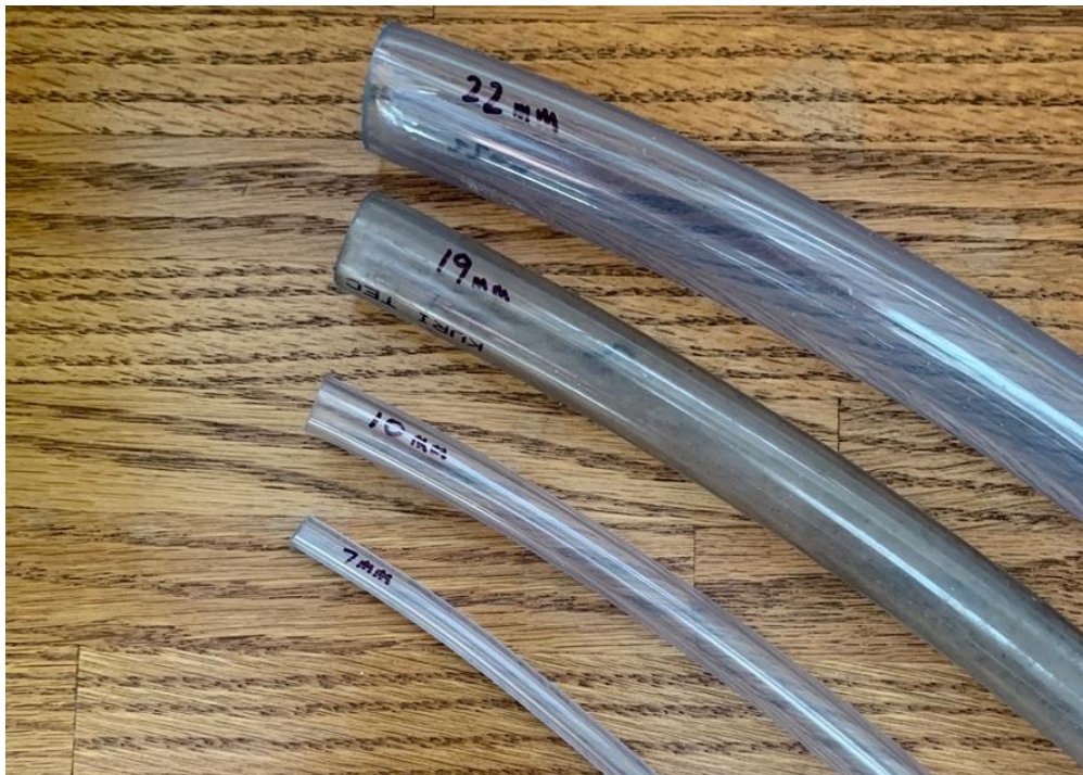
Figure S2. Plastic tubing used to measure the diameter and depth of interstitial refugia.
